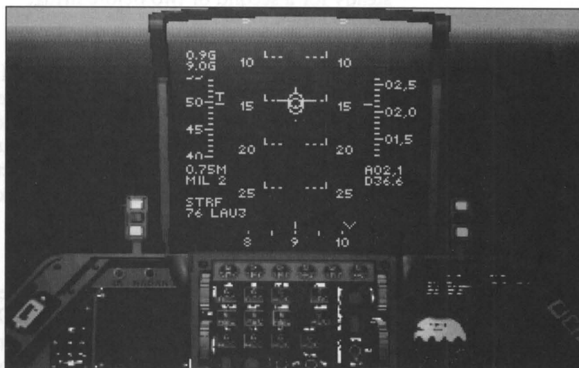
Figure 10-1 HUD prepared for a rocket strafing attack
