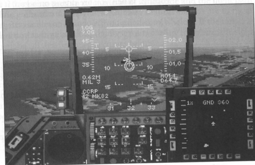
Figure 11-2 CCRP aiming sight on the HUD
