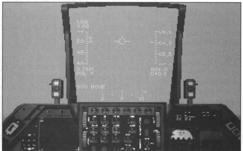
Figure 2-6 Velocity Vector Indicator within the HUD
