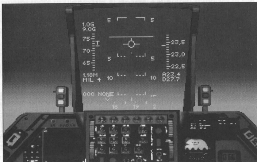
Figure 2-9 Velocity Vector Indicator and Pitch Ladder indicating negative pitch, or dive
