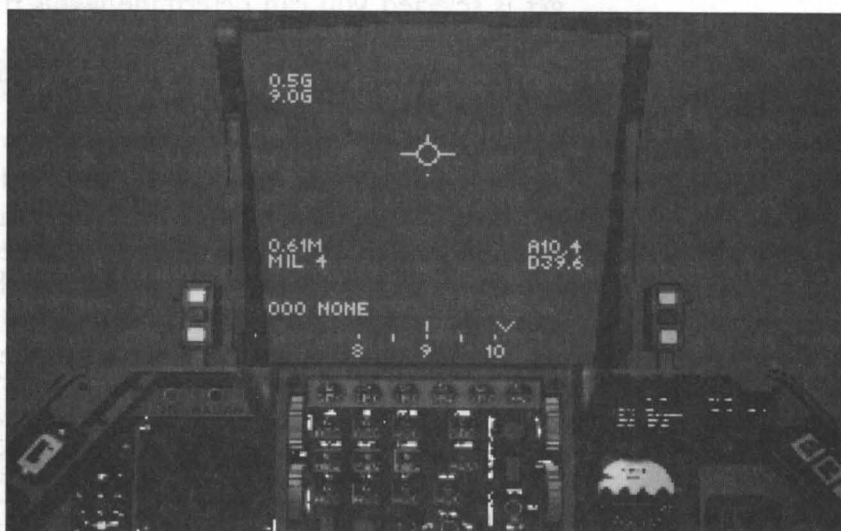
Figure 6-16 HUD with optional Airspeed and Altitude Tapes off
