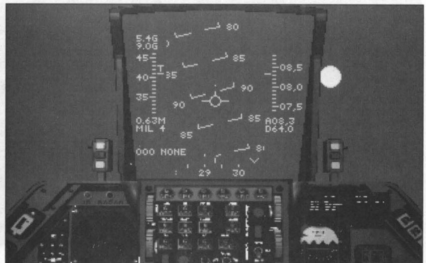
Figure 2-13. HUD G force readouts
